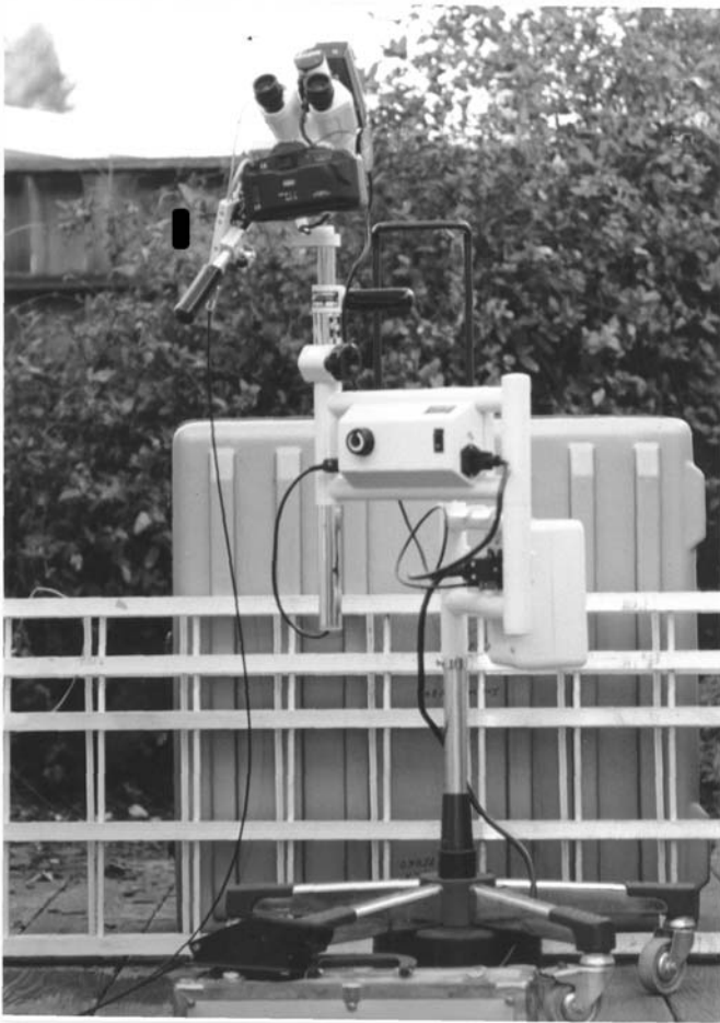
FIG. 1—SART-TO-GO-Mobile Colposcope Unit: colposcope with rolling base, hard travel-case, and folding motorcycle ramp, for loading. (Used with permission of CooperSurgical/Leisegang, Inc.)
